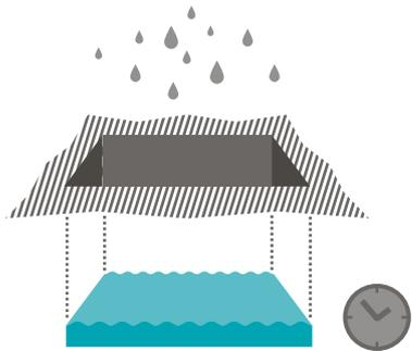
Because dry ground absorbs water more quickly than damp ground, the pit must be pre-soaked for about an hour. Only then will seepage be consistent and practice-oriented results be achieved. In this phase, the pit must not be allowed to dry out during soaking!
