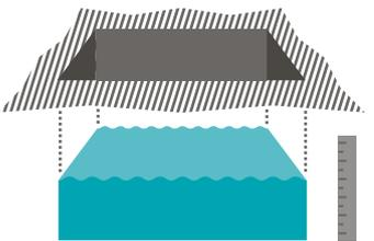
Once the ground has been thoroughly soaked, measurements can be made. The pit is filled with water and the water level and time recorded. At the end of this measurement, the time and water level are again recorded. Three measurements should be made consecutively. The pit can be refilled with water between two measurements as required.
