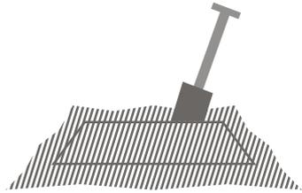
This requires a 30×30 cm square, pit that is around 30 cm deep. The bottom must be perfectly level. The bottom is covered with a 1 to 2 centimetre-thick layer of fine gravel to prevent mud from accumulating. It is important that the test be carried out at the depth at which the filtration system will subsequently be built.
